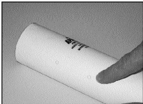
1. Peel backing from 'MULTI 2.75 ROCKET LAUNCHER BOLTS LOCATOR', and wrap around LAUNCHER TUBE aligning top and bottom rules. Trim tube to length of locator. Note difference in hole sizes on opposite sides.
