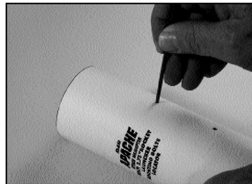
3. Clean holes using a small round file.
